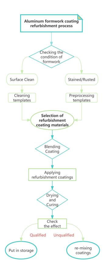
Aluminum formwork coating refurbishment process
